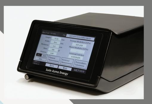
According to ASTM E1876, ISO 12680-1 and EN 843-2, it is possible to analyze the materials characteristics of homogeneous and isotropic objects with the standard shapes such as bars, rods, or discs.
